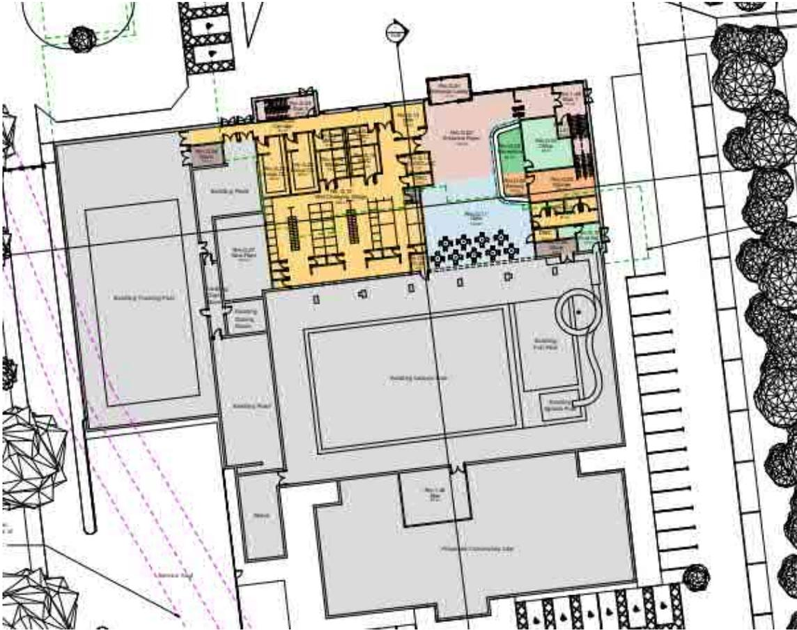
Figure 7 – Proposed First Floor Layout Plan
